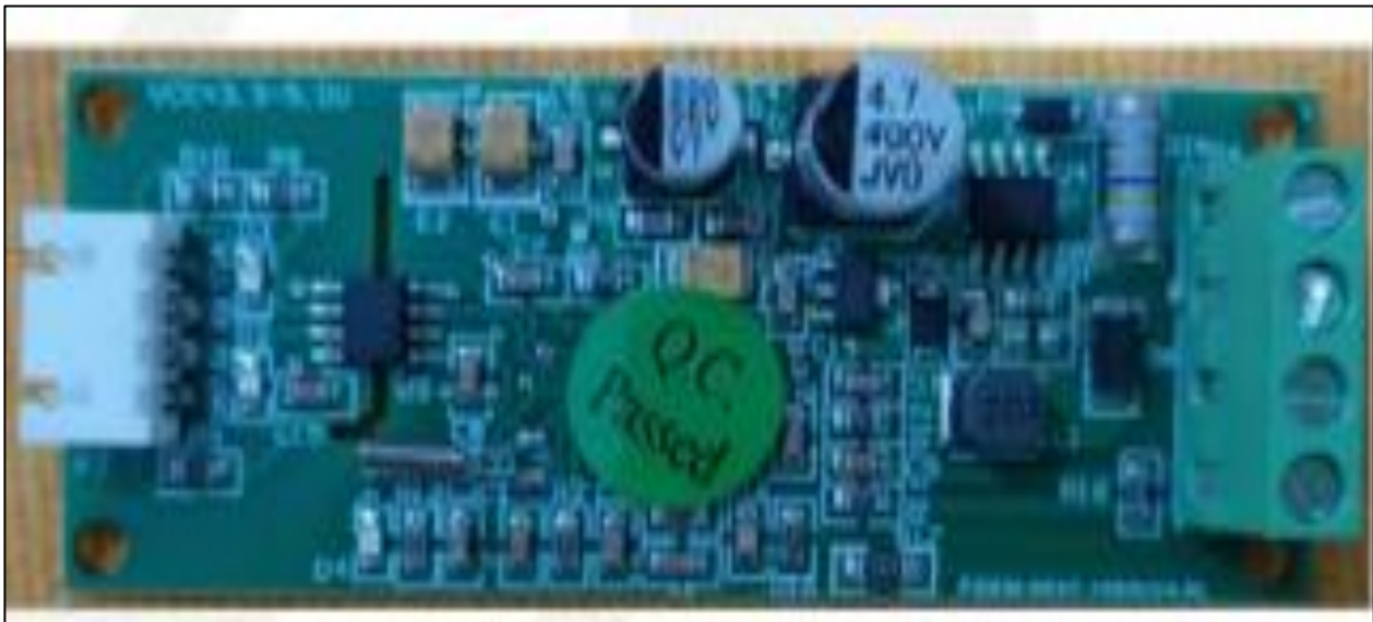
Figure 3: Voltage and Current Sensor Reading Circuit. Source: Authors, (2026).
