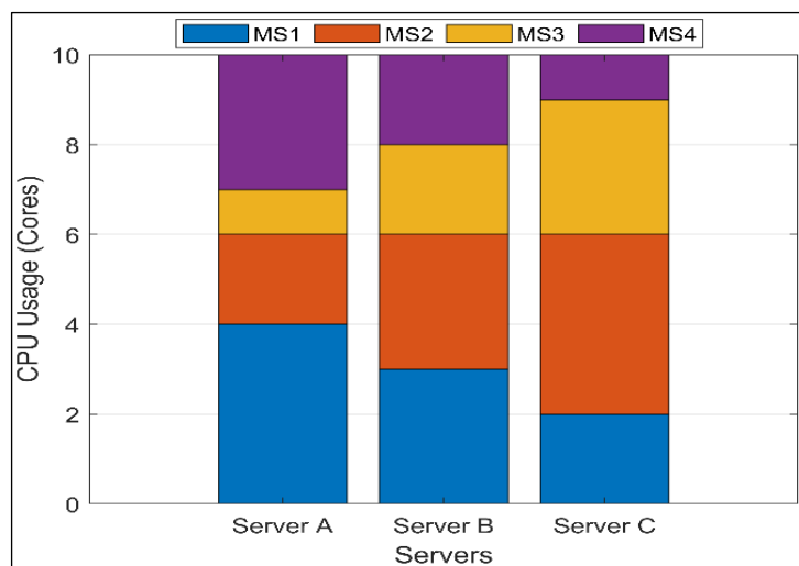
Figure 9: CPU Usage per Microservice across Servers.
