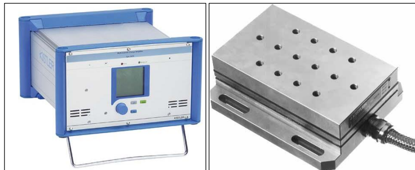
Figure 2: Force measurement aperture Kistler Type 5070A. Source: Authors, (2026).
