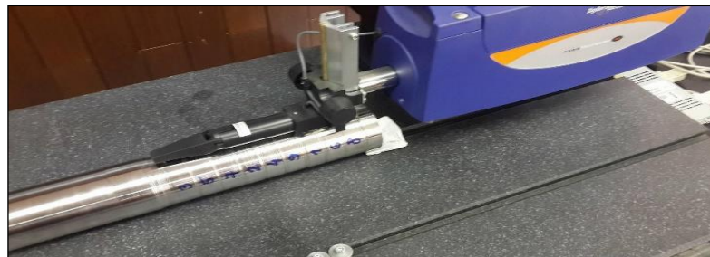
Figure 3: Measurement of surface roughness with TALYSURF, TAYLOR HOBSON. Source: Authors, (2026).
