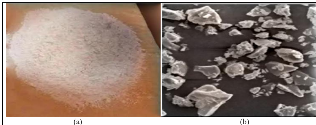
Figure 3: (a) Alccofine Normal View (b) SEM Analysis.
