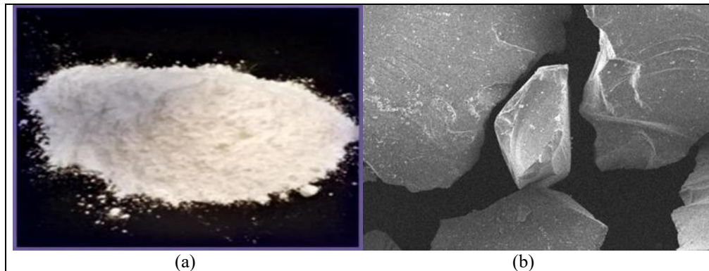
Figure 1: (a) Waste Glass powder (b) Waste Glass powder SEM Analysis.
