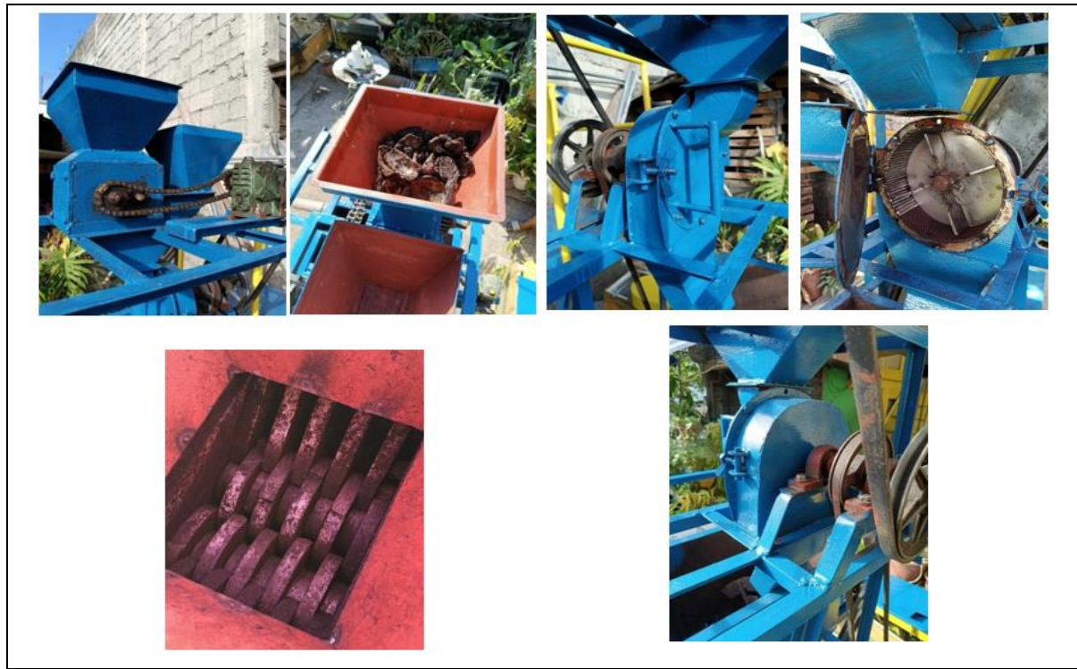
(a) (b) Figure 4: The two-stage pulverizer. (a) Knife-blade Shredder (b) Hammer Mill. Source: Authors, (2026).
