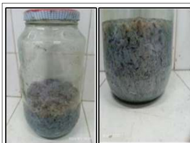
Figure 2: Experimental system used in the aqueous leaching test of leather shavings. Source: Authors, (2026).
