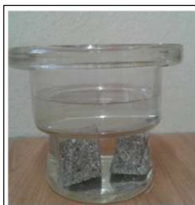
Figure 3: Experimental system used in the leaching test in the aqueous leaching test of the leather chips incorporated into the mixtures. Source: Authors, (2026).
