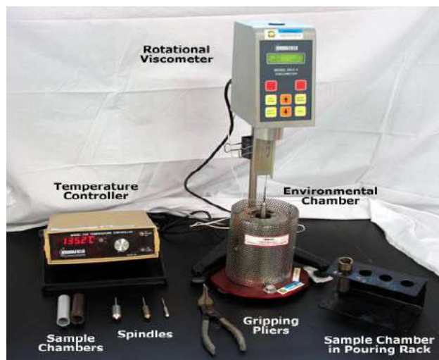
Figure 8: Rotational Viscometer, used for the Brookfield Viscosity Test. Source: [18].
