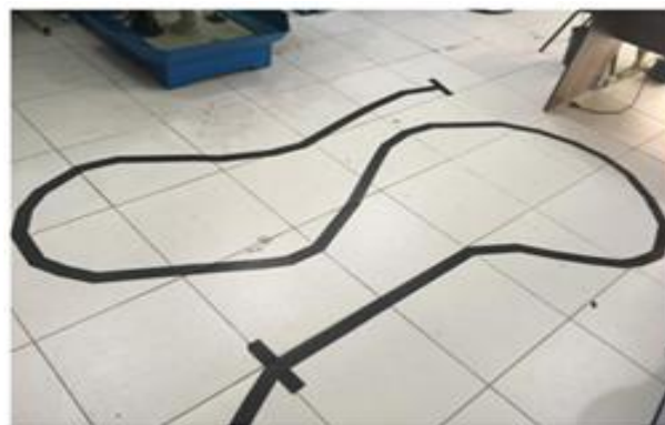
Figure 27: Demarcation for the robot to follow. Source: Authors, (2019).
