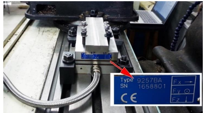
Figure 2: Dynamometer tag indicating F_x , F_y and F_z axes orientation.
