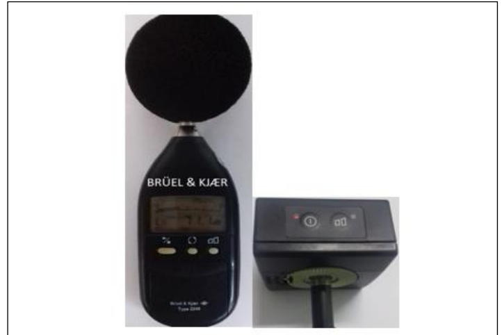
Figure 11: Sound pressure gauge (left side). Verification of the sound pressure gauge measurement (right side). Source: Authors, (2019).
