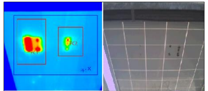
Figure 4: Cells with critical damage. Source: Author, (2020).
