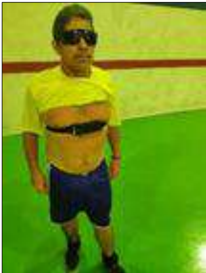
Figure 6: Elastic belt with vibrating devices placed in the athlete's chest position. Source: Authors, (2021).
