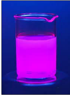
Figure 6: Rhodamine WT as a fluorescent dye substance. Source: Authors, (2021).
