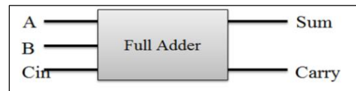
Figure 4: Schematic diagram of full-adder. Source: Authors, (2021).
