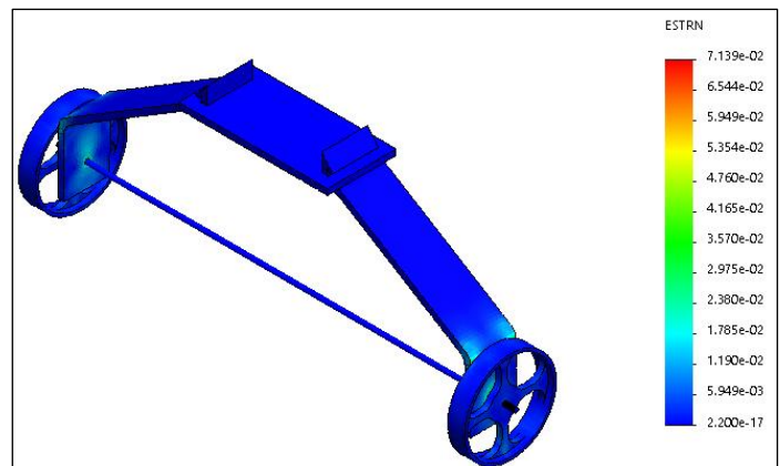
Figure 10: Result of deformation analysis in the Drop test. Source: Authors, (2021).
