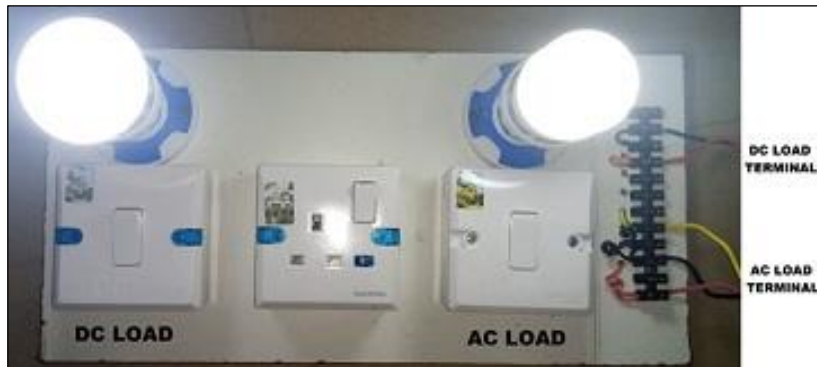
Figure 6: Hybrid Load on Wooden Board when Powered. Source: Authors, (2021).
