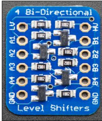
Figure 10: Bidirectional voltage converter. Source: Taken from [36].
