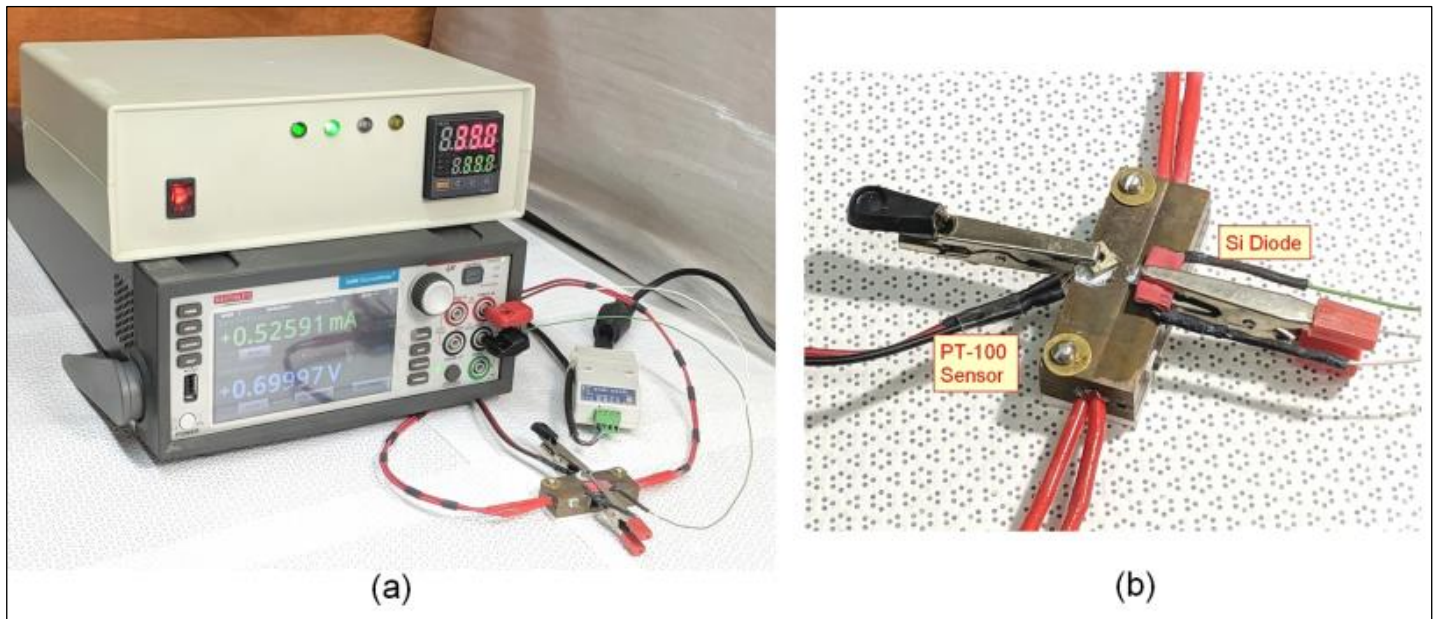
Figure 6: (a) Keithley Model-2450 Source Meter and heater power supply integrated with an Autonics TK series temperature controller connected via a USB-to-RS-485 converter. (b) View of the copper-made heating plate mounted with two cartridge heaters, one PT-100 sensor, and a common silicon diode IN-4007 as the device under test (DUT).
