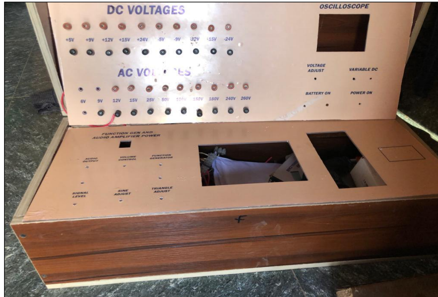
Figure 9: The smart electronic project lab casing. Source: Authors, (2023).
