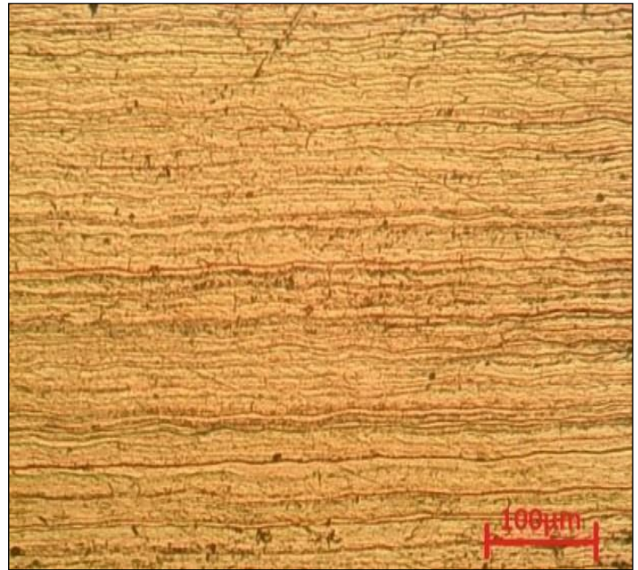
Figure 1.a: ASS-316 base metals' microstructure. Source: Authors, (2024).
