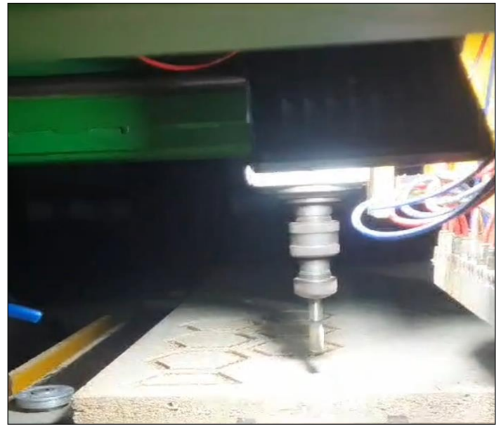
Figure 7: Drilling in the wood. Source: Authors, (2024).
