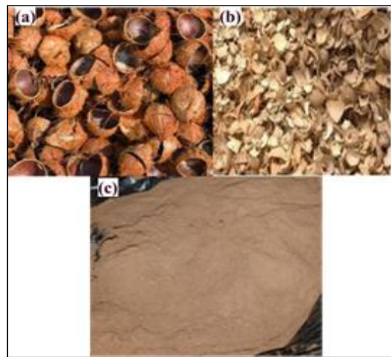
Figure 1: The reinforcing coconut shell organic waste (a) uncrushed (b) crushed, and (c) powder.
