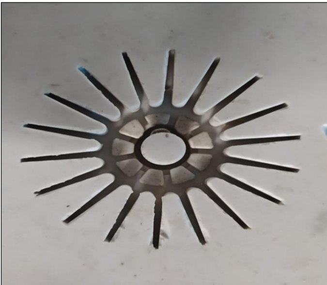
Figure 3: Impeller mold. Source: Authors, (2024).
