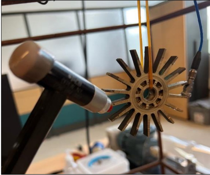
Figure 6: Dynamic vibration test on blades. Source: Authors, (2024).
