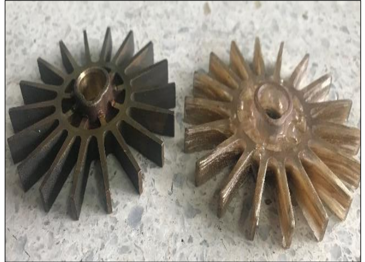
Figure 4: Fabricated impeller and conventional impeller. Source: Authors, (2024).
