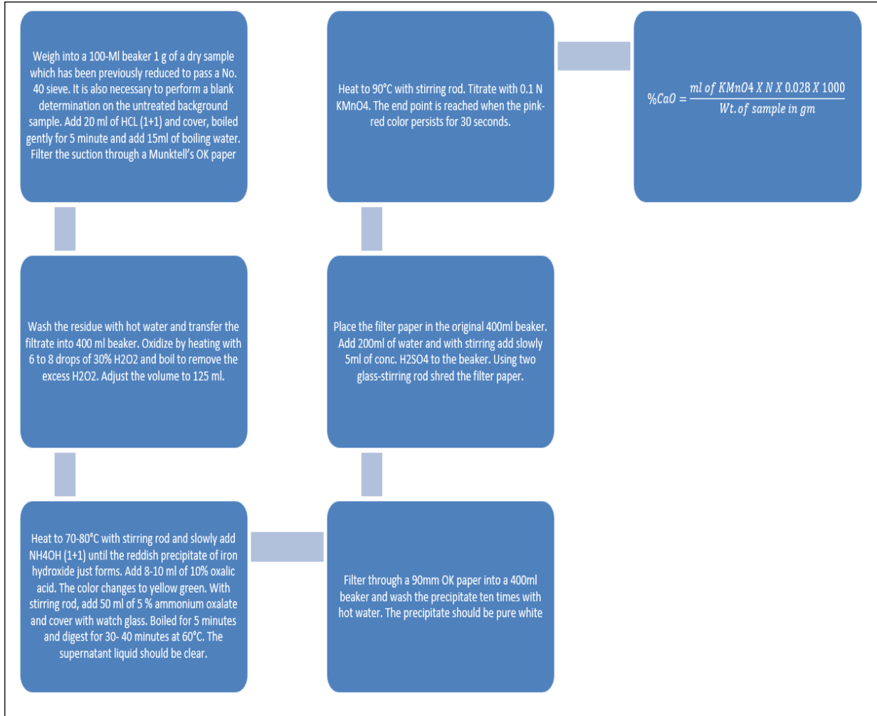
Figure 1: California Test 403 Procedure. Source: Authors, (2023).
