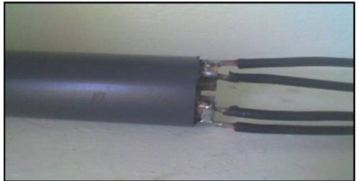
Figure 11: Augmented Rail Launcher Wiring.
