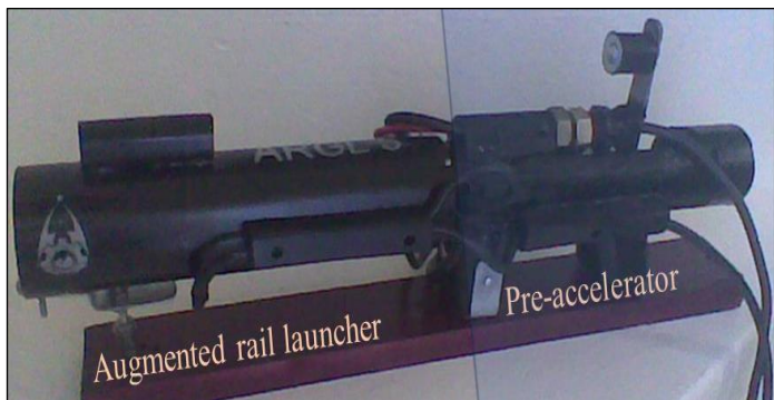
Figure 13: Final assembly of the augmented rail launcher. Source: Authors, (2024).
