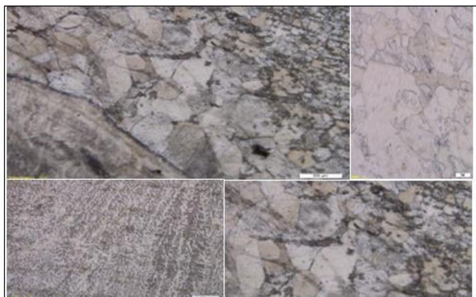
Figure 113: Sample welded at a heat input of 1.75 kJ/mm. Source: Author, (2024).
