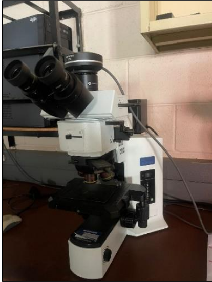
Figure 4: BX51M Olympus optical microscope Source: Author, (2024).
