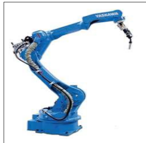
Figure Error! No text of specified style in document.: Yaskawa robotic welder. Source: [21].
