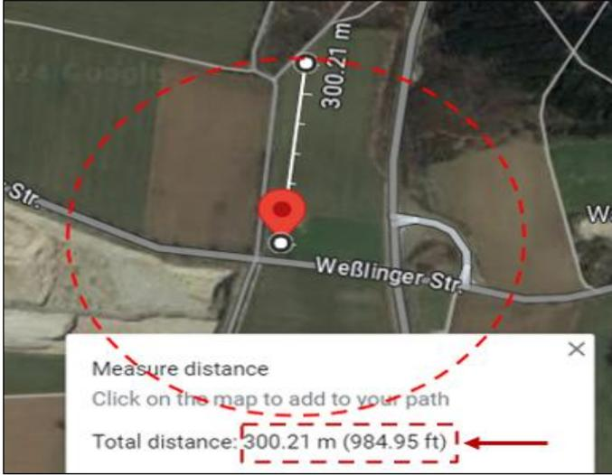
Figure 6: Setting the radius of Geofence circle.
