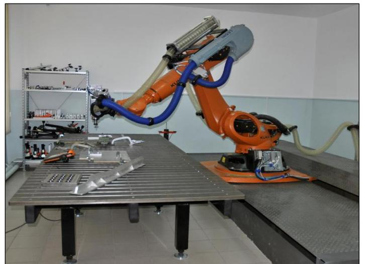
Figure 9: Robotic complex based on KUKA KR 210 R2700 EXTRA industrial robot.
