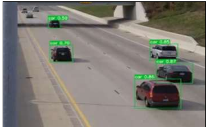
Figure 2: Real-time Vehicle Detection via YOLOv7.
