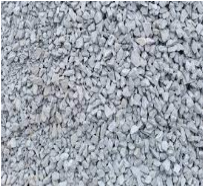
Figure 9: Coarse aggregate (Granite) Source: Authors, (2025).
