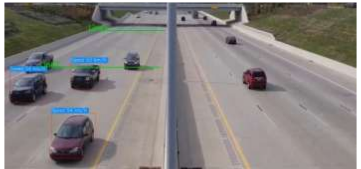
Figure 7: Simultaneous Detection, Tracking, and Speed Estimation of Multiple Vehicles.
