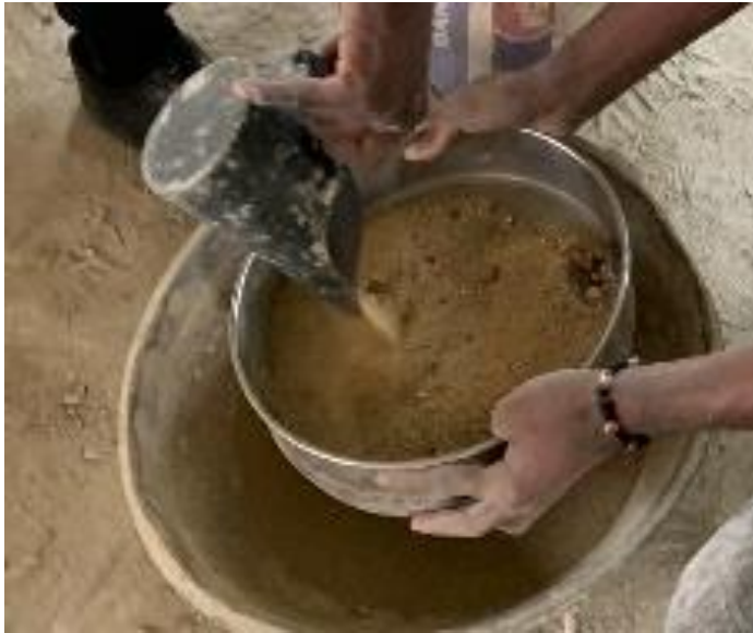
Figure 8: Sieving of fine aggregate (sand). Source: Authors, (2025).
