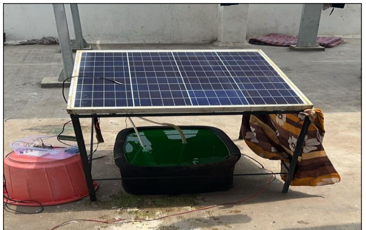
Figure 5: Wet Testing Setup with Ethylene Glycol. Source: Authors, (2025).
