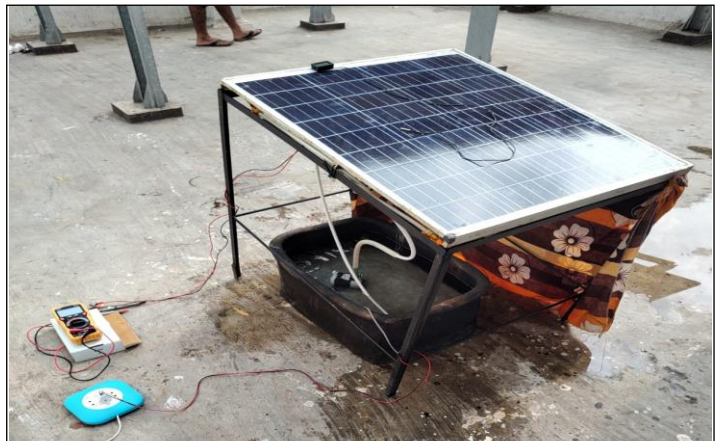
Figure 4: Wet Testing Setup with water Source: Authors, (2025).
