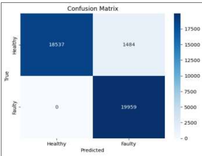
Figure 5: Confusion matrix of LSTM for vibration dataset. Source: Authors, (2025).
