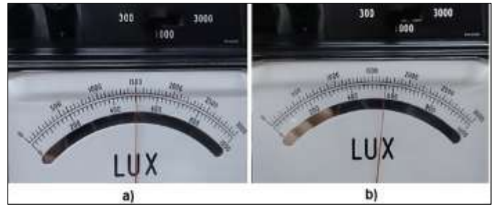
Figure 3: Comparison of the light level on the work plane, a) fluorescent tube, and b) LED tube.
