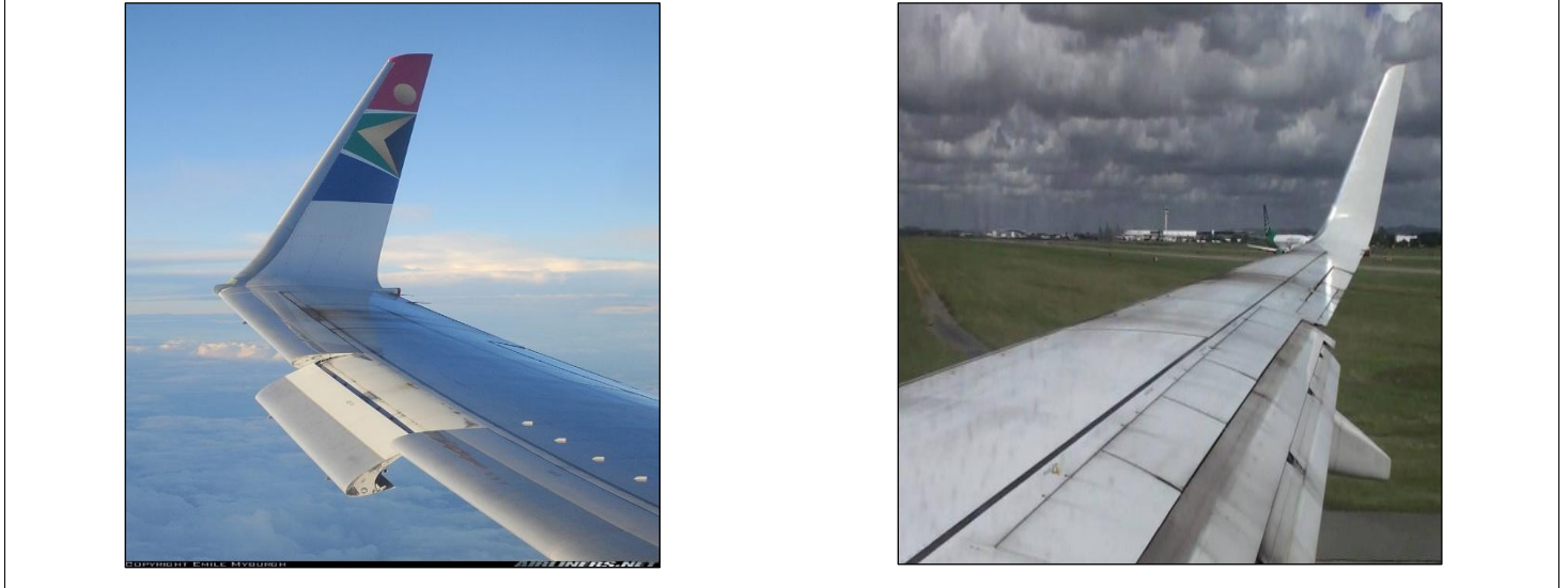
Figure 3: Leading edge slot and trailing edge flap.
