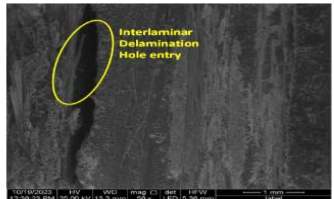
Figure 6: SEM Image for frontal plane hole entry at 56 X Source: Authors, (2026).
