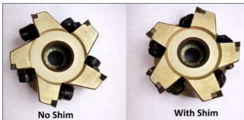
Figure 5: 63mm Diameter Face milling tool with 5 inserts. Source: Authors, (2026).
