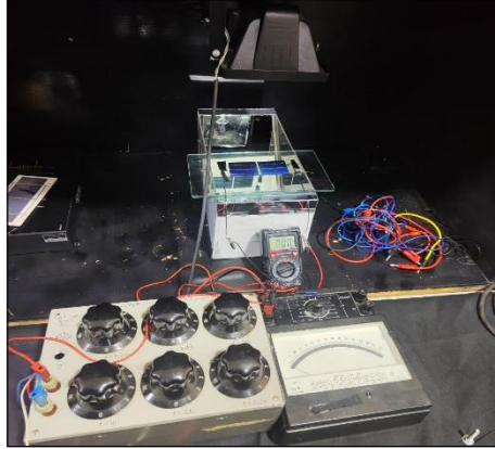
Figure 4: The circuit assembled for experimental measurement of the I – V characteristics. Source: Authors, (2026).
