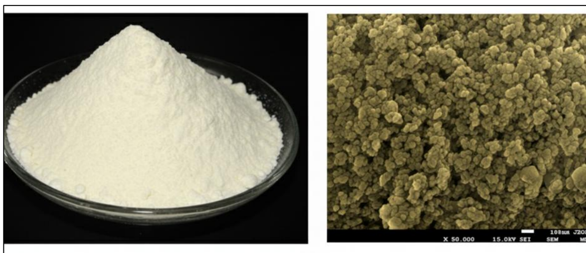
Figure 1: CeO 2 Nanoparticles – Powder & SEM Morphology.
