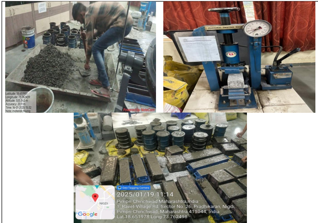
Figure 14: Preparation of concrete specimens in the laboratory. Source: Authors, (2026).
