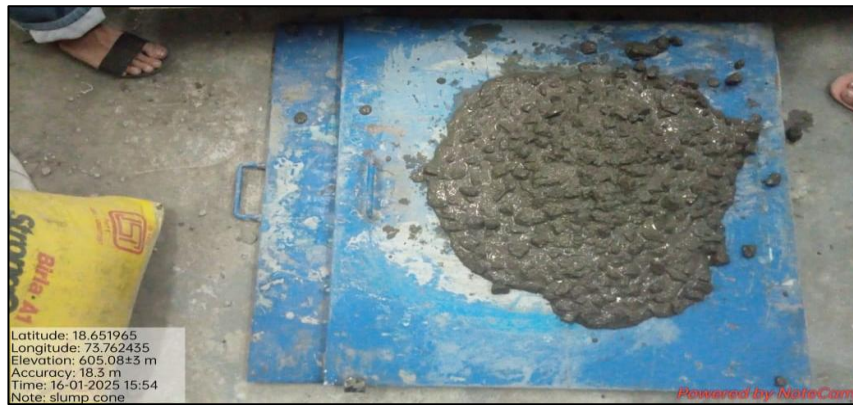
Figure 7: Flow Table Test Performance.
