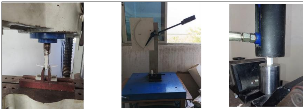
Figure 1: Flexural, Impact and Compression testing setup
