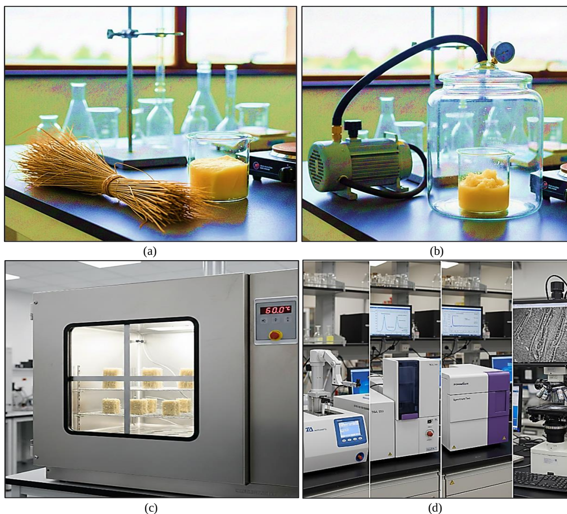
Figure 1: Schematic overview of the experimental methodology. (a) Pre-treatment of raw materials: thermal purification of animal fat and alkaline modification of Stipa ichu fibers. (b) Bio-composite synthesis via vacuum impregnation to ensure capillary infiltration. (c) Accelerated thermal aging protocol illustrating the temperature cycling profile. (d) Summary of physicochemical characterization techniques employed.
